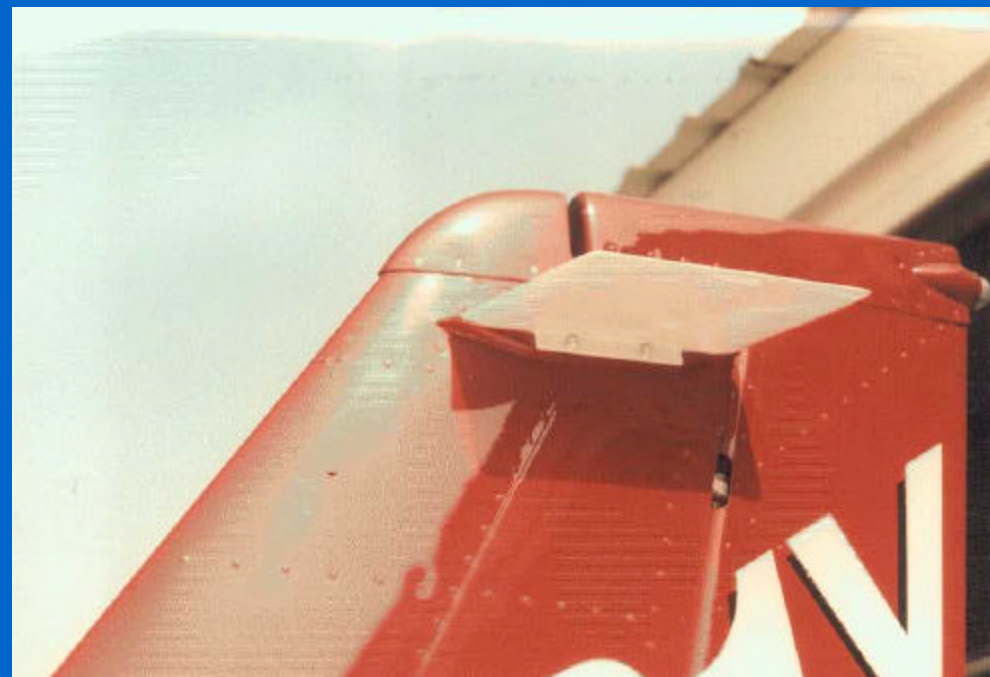
K2U Fin Cap - Strobe in Rudder
