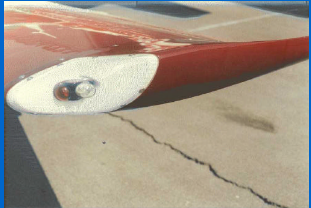
Johnston Wingtips with Enclosed Lights
