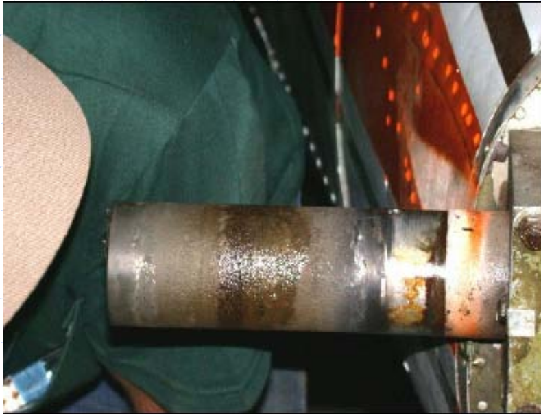
Typical Severe Corrosion On Torque Tube
