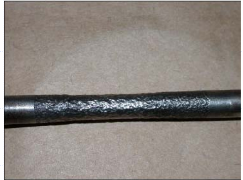
Typical Corrosion on AN5 Bolt Holding Horn to Torque Tube
